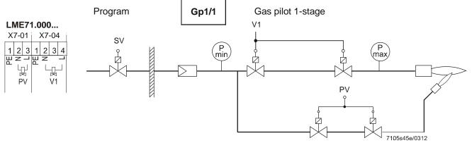
Figure 3: Fuel train gas pilot ignition 1 (Gp1/1), 1-stage
