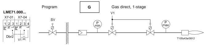
Figure 2: Fuel train gas direct ignition (G), 1-stage
