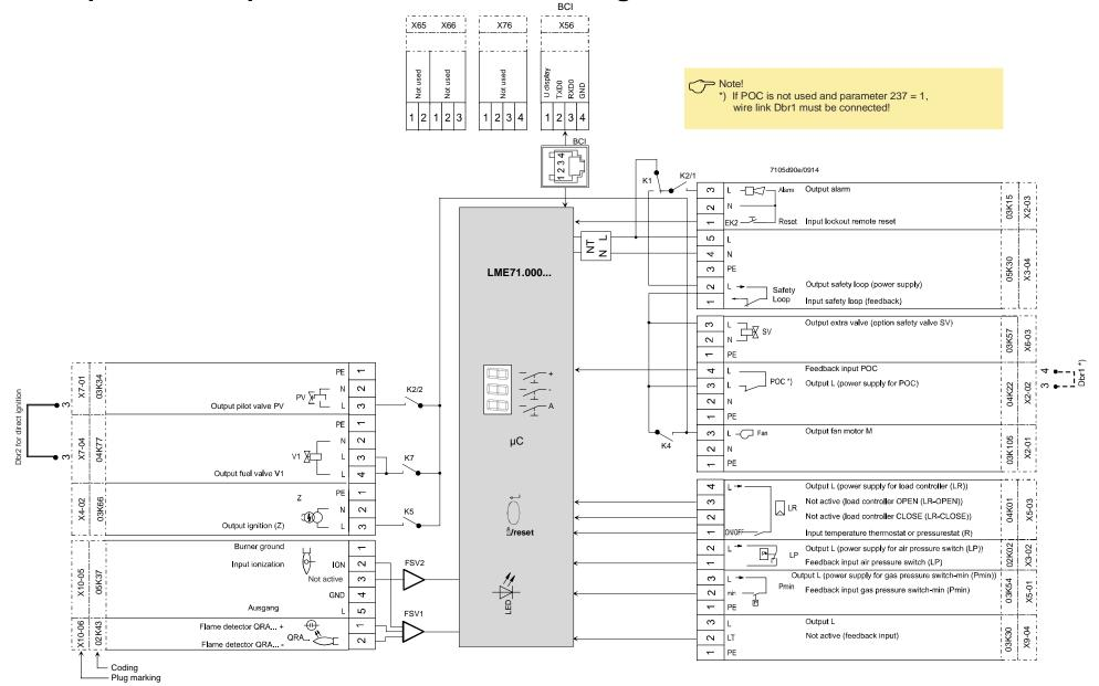
Figure 4: Inputs and outputs / internal connection diagram
