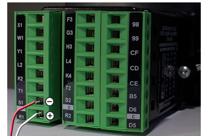
Figure 4: Thermocouple Wiring Example
