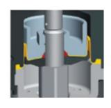
The NGRB2 and NGRB3 pressure regulators have an internal balanced valve allowing low lock up even with high inlet pressure variations. Due to its ruggedness and simplicity, the maintenance is fast and easy. Due to its top entry design, it is not necessary to take the body out of installation to be repaired.
