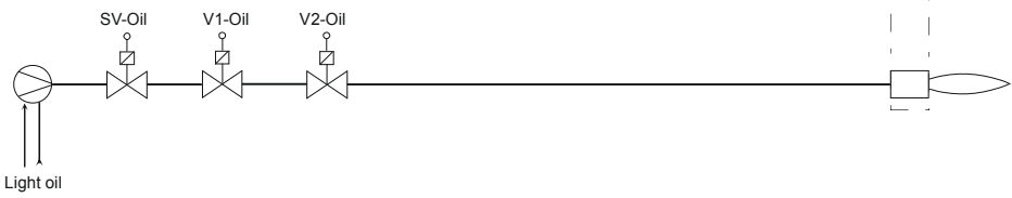
Figure 60: Dual fuel burner gas / light oil with gas pilot ignition, with 2 fuel valves
