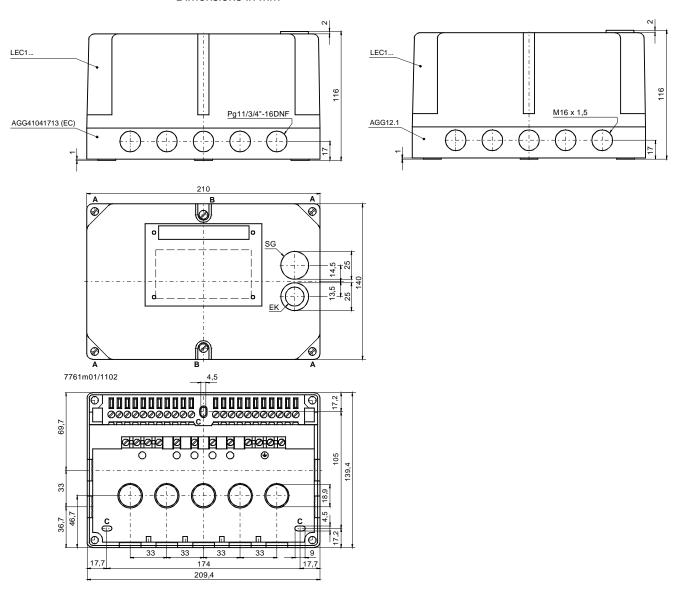
To remove the control unit from the plug-in base, loosen **only** the 4 screws  $\bf A$ . To remove the unit cover, also loosen the 2 screws  $\bf B$ .
