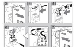
Set the solenoid actuator to the correct position again and screw the hexagonal nut/cap tight if applicable.
