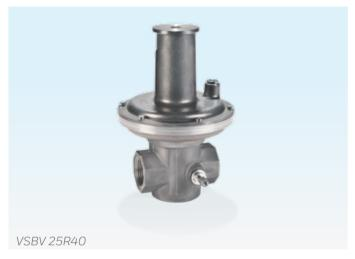
Safety relief valve for relieving brief pressure surges in control systems thus preventing the safety shut-off valve JSAV from being activated unintentionally. The VSBV reduces too high a pressure increase due to gas creeps which are the result of gas pressure regulators that are not tight closing.
