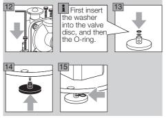
Replace the O-rings on the housing and the valve seat.
