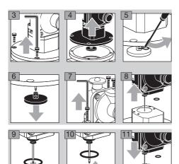
Ensure that the O-ring is fitted in the new measuring unit, see Figure 11.
