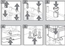
The cylinder pin in the drive shaft must be locked in the coupling.
