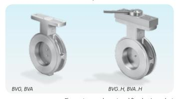
Flow rates can be set and fixed using a butterfly valve with manual adjustment, for example to limit the high-fire rate on the burner. A scale indicates the set angle of opening. Butterfly valves BVG, BVGF, BVA and BVAF with reduced nominal diameter (reduced by one or two nominal sizes) can be used to achieve higher control accuracy. This will mean that complex reducing fittings will no longer be required.
