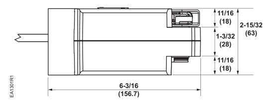
Figure 14. GQDxx6 with Conduit Adapter.
