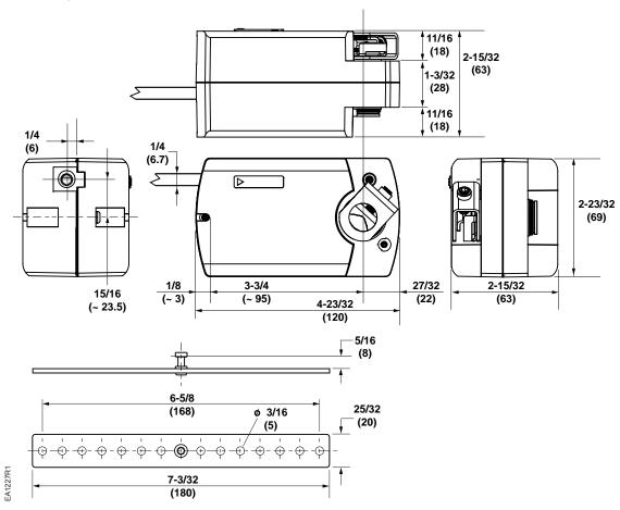
Figure 12. GQD1x1 Actuator and Mounting Bracket.
