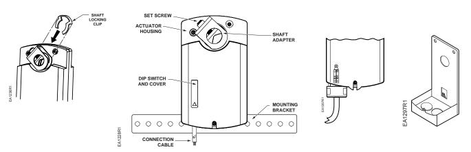
Figure 1. Components of the GQD Spring Return Actuator.
