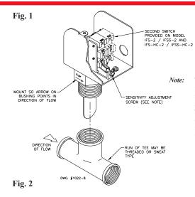
Turn screw clockwise to increase the flow rate required to activate the switch. Turn screw counterclockwise to decrease the flow rate required to activate the switch.
