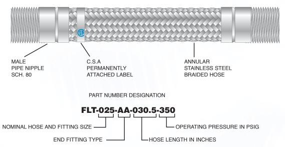
EXAMPLE: The above part number designation is for a 1/4" size hose with a SCH 80 Steel Male Nipple on each end, 30.5" long, working at an operating pressure of 350 PSIG.
