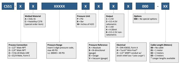
Ordering Example: CS51-2A00010PG4H000-00 (1/4" Male NPT, 316L SS, 0-10 PSI gauge, 4-20mA, Turck® Mini-Fast®)
