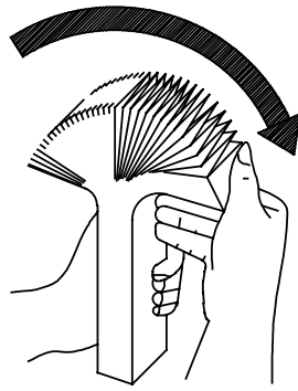
Fig. 5.5 Loosening the Chart Paper
