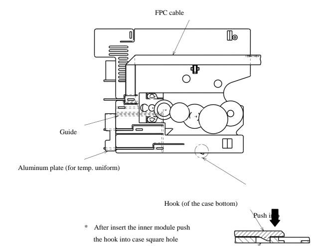
6. After installation make sure, by opening/closing the door, FPC cable will smoothly slide in a space between case and inner module. If not slid well, please reinstall inner module again.
