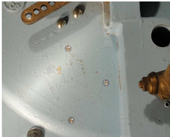
Figure 4: Drawer with Holes Marked and Started
