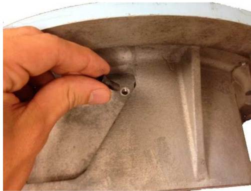
Figure 14: Remove Mechanical Stop Screw for SQM33 Actuator
