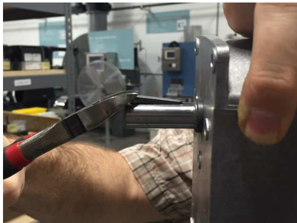
Figure 2: Removing the Key from an SQM48... Actuator
