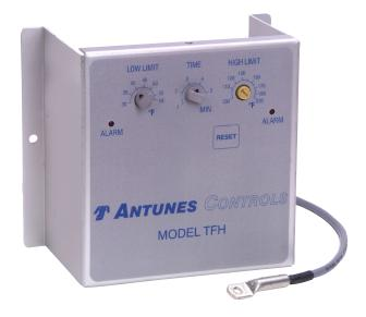
The TFH is a three-in-one freezestat that incorporates a temperature monitor, delay timer, and high-limit controller into one compact and conventional unit. It is typically used in air make-up equipment. The low limit monitors the temperature to the desired setpoint and will shut down the system if the setpoint if not achieved by the setpoint time. The high limit monitors the temperature and will shut down the system if the temperature exceeds the setpoint.
