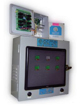
The ACME CEL(LS) MultiSet series is a microprocessor-based multipoint multigas detection and control system that can be used with a wide variety of ACME toxic, combustible, refrigerant & oxygen gas sensors. The sensors can be grouped in any combination. The wiring between the Control Panel and the remote sensor-transmitters is accomplished via 4-wire "low voltage" "daisy-chain".
