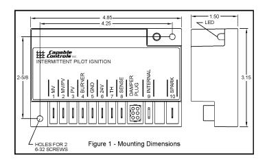
The high voltage spark cable should be of the noise suppression type rated for at least 15kV and must not be in continuous contact with a metal surface. If separate flame sense probe is used, the sense wire must be separated from the high voltage wire by a minimum of 1/4".
