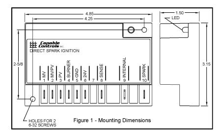
Power must be provided from a properly sized 24 volt class 2 transformer. All wiring must be done in accordance with both local and national electrical code. All wiring and initial operation must be performed by a qualified service technician.
