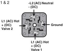
Procedure for Testing Valve #1
