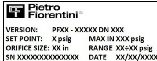
Figure 10: Equipment rating plate
