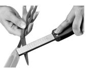
at the point where the bevel reflects most brightly. Drag the two-sided pocket sharpener up the length of the scissor blade from hinge to point. It may be helpful to use the marker method described in the **Sharpening Knives** section to make sure the entire length of the blade is sharpened. Once one blade is sharpened, flip the scissors over and repeat the procedure on the second blade.
