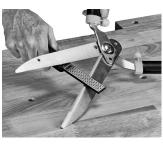
brightly. Drag the two-sided pocket sharpener up the length of the shear blade from hinge to point. It may be helpful to use the marker method described in the Sharpening Knives section to make sure the entire length of the blade is sharpened. Once one blade is sharpened, flip the shears over and repeat the procedure on the second blade.
