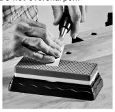
After a light burr forms on the cutting edge, drag once over the fine stone to remove.
