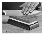
pen before pulling the knife across the stone. If the knife was held at the proper angle, the marker color will be gone. If any marker remains, try sharpening again
