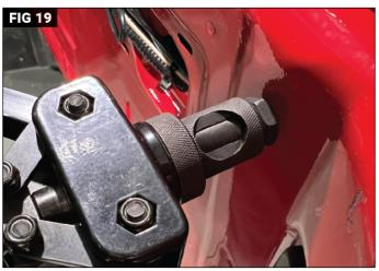
Start with a smaller bit than needed, to drill four pilot holes. Use the full-size 3/8" bit to open the hole to the correct size for the Rivet Nuts (Fig 18). (This can be done with a step bit, as well). Using a Rivet Nut tool, insert a Rivet Nut fully into each of the four holes. (Fig 19) Replace the rear plastic trim piece by inserting the upper tabs first. Then, press in the clips along the bottom.
