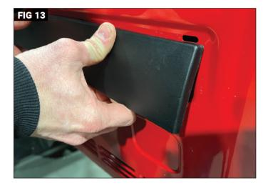
Put on safety glasses. Removing the rear tailgate trim piece makes the marking and drilling easier. The trim can be removed by carefully working a trim removal tool or fingers, starting on the bottom left corner. Carefully work under that corner and slide to the left, releasing the clips as you go. (Fig 13) Once all the lower clips have been released, lift the lower portion and pull forward to release the upper tabs from the slots.
