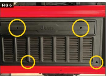
The smaller trim piece has two drill points marked inside two circular raised locations. Drill the holes there. (Fig 5) These line up with the two mount points shown in previous step. (Fig 3) When the trim pieces are reinstalled, there should now be 4 drill holes present to correspond with the marked mounting points from step 2. These are marked with a yellow circle. (Fig 6)
