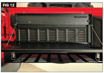
Close the table and secure the latches. Insert the remaining two M6 button head bolts through the M6 flat washers into each of the lowest holes along the bottom of the back frame and into the spacers. (Fig 11) Tighten all four M6 button head bolts securely. **Note:** Do NOT over tighten bolts. The rivet nuts may begin to spin or pull out if overtightened.
