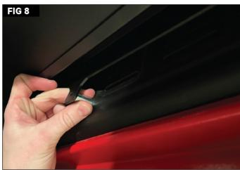
Place the 7mm spacers in the drill holes. The longer 33.5mm spacer should be placed in the lower right position. The three 30.5mm will be pushed into the other three locations. (Fig 7 & 8)
