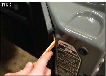
Put on safety glasses. There are two trim pieces on the rear tailgate that need to be removed. The first smaller trim can be removed by careful working a trim removal tool on one side and working around the edges, releasing the clips as you go. (Fig 1) Set this piece aside for use in Step 3. Using the trim removal tool, carefully remove the larger trim piece to reveal the entire framing and mounting points in the tailgate. (Fig 2)
