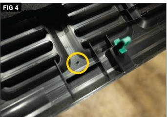
The four mounting points for the tailgate table are shown with the yellow circles for reference of all of the holes need to be drilled in each trim piece. (Fig 3) The lower two are used for the larger trim piece. There are two pre-marked drill points on the back of the larger trim piece to match the location of those mount points. Using the drill and 1/2" bit, carefully drill a hole at each of those two drill points. (Fig 4)
