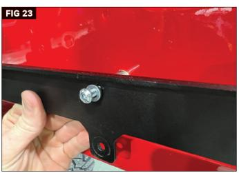
Install the 30.5mm spacer on the upper left corner and lower left mounting hole. (Fig 22) Place an M6 flat washer on the outside of the frame and loosely thread the M6 Button Head Hex Bolt into the spacer and Rivet Nut. (Fig 23) Use the longer 33.5mm spacer for the lower right mounting location. Place an M6 flat washer on the outside of the frame and loosely thread the M6 Button Head Hex Bolt into the spacer and Rivet Nut. Do not fully tighten at this time.
