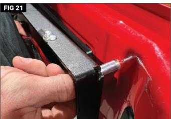
Check that each rivet nut is fully seated and secure. (Fig 20) Starting on the upper right corner near the Quadratec logo, install the 30.5mm spacer between the back frame and the tailgate. (Fig 21) Place an M6 flat washer on the outside of the frame and loosely thread the M6 Button Head Hex Bolt into the spacer and Rivet Nut. Do not fully tighten at this time.
