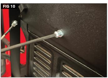
Hold the tailgate table in the open position against the tailgate and align the upper mounting holes to the mounting points with the spacers inserted. These mounting holes are just above the large opening in the back frame. Insert two of the M6 button head bolts through the M6 flat washers into each of these holes and into the spacers. (Fig 9 & 10) Do not fully tighten at this time.
