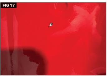
Using your free hand or a helper, locate the center of the flat portion of the tailgate by measuring this area and find the halfway point. This will help make your marking more accurate. Then, hold the back frame level against the tailgate and mark the locations that need to be drilled. (Fig 16) Use a center punch to make a dimple to start the drilling process. (Fig 17)
