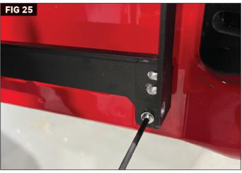
Using a 4mm hex wrench, tighten each of the four button head bolt to secure the frame to the tailgate. (Figs 24 & 25) **Note:** Do NOT over tighten bolts. The rivet nuts may begin to spin or pull out if overtightened.
