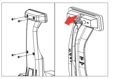
4. Attach Accessory Brake Light LED Ring to tire mount by sliding over mounting holes.
