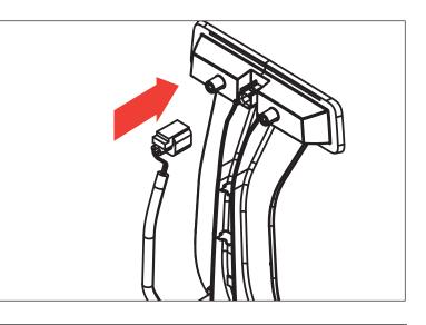
8. Reattach factory third brake light to factory tire mount.
