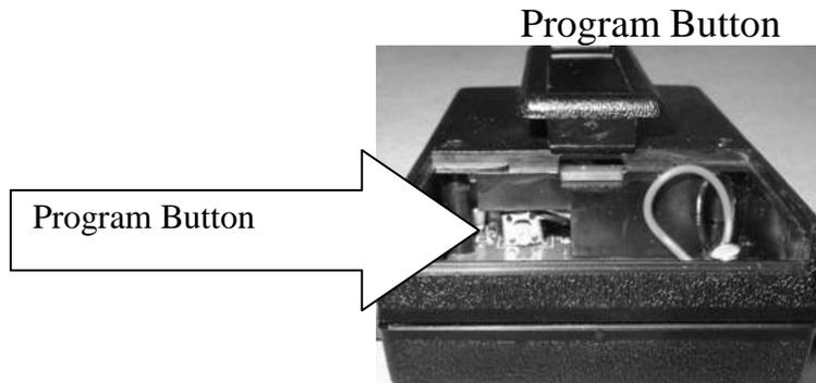
3. Press and hold the PROGRAM button in. While pressing and holding the program button, turn the Vibra-Call on, continue to hold the program button on for 8 – 10 seconds and then release it. This will erase all codes in the Vibra-Call memory.
