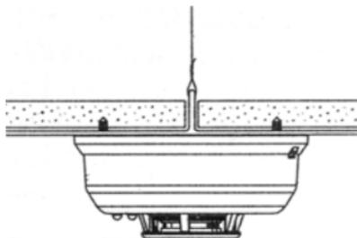
**Figure 9:** Mount Detector Across Ceiling Panel Support.
