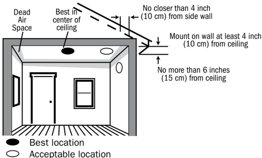
**Figure 4:** recommended smoke detector mounting locations.
