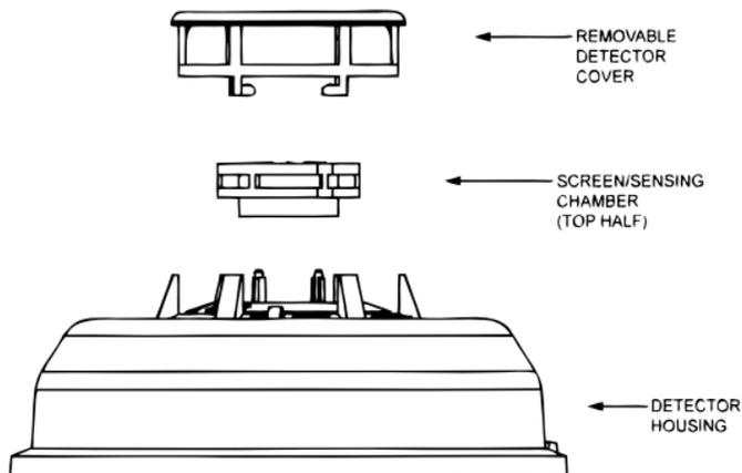
**Figure 11:** Removing Screen/Sensing Chamber
