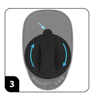
Place the powder container lid on the powder container and turn clockwise until it stops.
