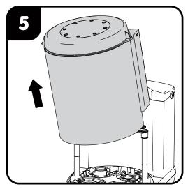
Remove wash compartment by lifting straight up.
