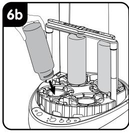
Narrow neck bottles can be placed through the center rings on the bottom rack.
