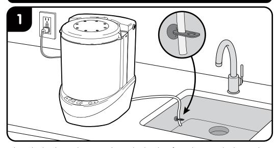
Place the bottle washer on a clean, dry, level surface close to a kitchen sink. Connect one end of drain hose to back/bottom of unit, secure the other end of the drain hose to the sink wall with the drain hose holder. Make sure the drain hose is aimed downwards or at the sink drain. Plug power cord into an electrical outlet away from water source.
