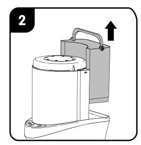
Remove water tank lid and pull the water tank up by the handle.
