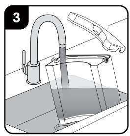
Fill the water tank with clean TAP WATER to the max line.
