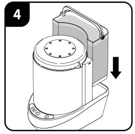
Place filled water tank back onto the base and replace the water tank lid.
