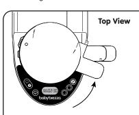
To place lid on bowl, position the lid as shown above, then rotate lid counter-clockwise. Make sure tabs on cover align with slots on front of bowl, handle and base of machine.
