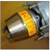
Slide the long clutch onto the engine crankshaft until the back of the clutch touches the shoulder of the crankshaft. Tighten the grubscrew and then the locknut.
