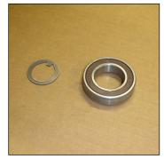
Remove the adapter flange from the engine. Remove the bearing from the flange. Refit the flange to the engine. The washer and bearing are no longer required and can be disposed of.
