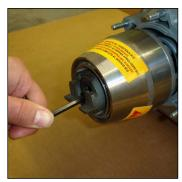
Undo the bolt in the middle of the clutch 2 to 2½ turns. Use the CORRECT size allen key: GX240/270 engine - ½ allen key GX340/390 engine - 7/32 allen key
