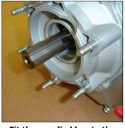
Fit the supplied key to the crankshaft.
