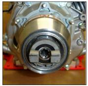
When the engine is refitted ensure that the two prongs on the front of the clutch are at the bottom to ensure the correct operation of the clutch.
