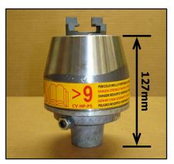
If your clutch is held onto the engine's crankshaft by a locking nut and grub screw on the back of the clutch and measures 127mm, then follow step 3.
