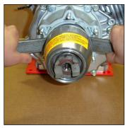
Carefully pry the clutch from the crankshaft. Once the clutch has released from the crankshaft, fully undo the bolt in the centre of the clutch and remove clutch.
