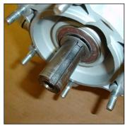
Remove the washer from behind the clutch.
