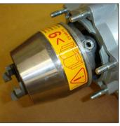
Remove the clutch from the crankshaft by undoing the locking nut and grubscrew.
