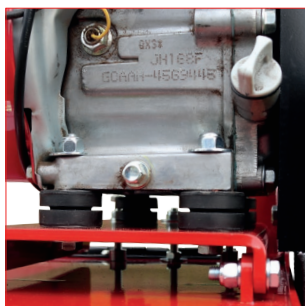
RUBBER MOUNTS Engine fitted to rubber mounts to reduce vibration.
