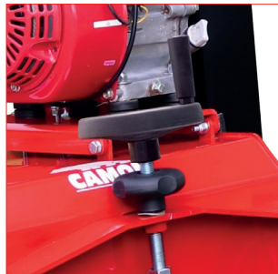
FINE HEIGHT ADJUSTMENT Lockable, precise height adjustment.
