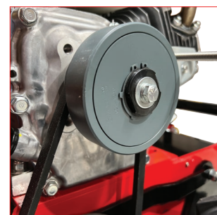
CENTRIFUGAL CLUTCH For operator safety and reliable performance.
