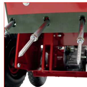
SELF-PROPELLED The action of the tines walks the machine forward.
