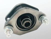
There are two types of coupler - the old machine to new implement coupler converts the spline shaft of an older power unit so it can operate the current implements with the 3-dog coupling, or the new machine to old implement coupler allows old implements to be used on new power units.
