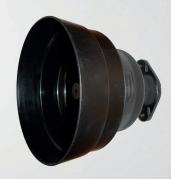
The Tractor PTO Coupler converts the BCS PTO to a 6-spline allowing the power unit to operate certain low power, stationary implements. It is important to note that the the BCS power units run at 990rpm.
