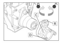
To fit and remove the Lawn Scarifier simply rotate the knob (Fig 3,R). The device is locked by turning the knob clockwise and unlocked by turning the knob anticlockwise. It is important that nuts (Fig 3,D) are well tightened.
