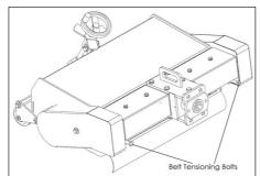
Remove the gearbox frame covers by undoing the two bolts holding each cover onto the gearbox frame.
