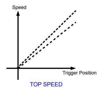
Turning the Pot fully clockwise is Top Speed Anti-clockwise reduces it and limits the speed
