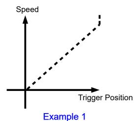
End Sensitivity set to Minimum Shows the largest final step and reduced Speed for the rest of the response line.
