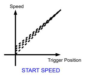
Turning the Pot clockwise increaces The Start-up speed. Anti-clockwise reduces it.
