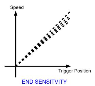
Turning the Pot clockwise increases the end speed and reduces the size of the final step. Anti-clockwise is the opposite.
