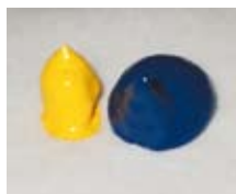
Incorrect ratio mixing
