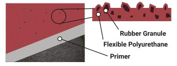
This system is comprised of combining a resilient EPDM granule with a flexible water-based polyurethane coating system. The granule provides anti-slip properties but with a softer feel to bare feet.
