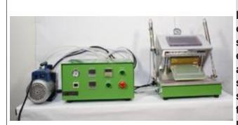
PC-FVS is a pouch cell vacuum sealing machine. This operation is done in dry atmosphere. After the cell is sealed two sides, then electrolyte is added. The the electrolyte is diffused properly using PC-AD and the air bubbles are removed. Then the final vacuum sealing is done. This unit consists of three parts, sealing, controller and vacuum pump. Sealing temperate and the time can be adjusted. Compressor need to be connected for the operation of the sealer.
