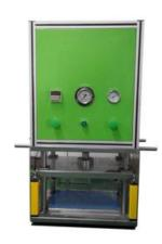
PC-EP is a pouch cell electrode punching machine. Both cathodes and anodes can be punched using this machine. This is a semi-automatic machine once the electrodes are fed the cutting/punching action is done using a foot pedal. The die has to be matched with that of the case forming machine PC-FM. There is a built in IR sensor safety feature for safe operation of this unit. Optional different size dies are also available.
