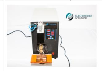
CC-SWM is a precise single point pneumatic welder designed for Itihium ion battery cyclindrical cells to weld anode and cathode. This is designed for small volume R&D labs. 2mm x 180mm length welding needle can be easily inserted into the cylinder case to weld at the bottom. Available in both 220V and 110V input voltages. Small size and light weight and can be operated with foot pedal. May need some practice to perfect it. Optimal welding conditions provide perfect welding.
