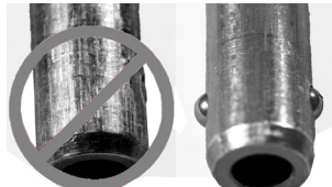
Fig 18 Left pin – retired due to wear and detent pins not properly working; Right pin – in good working condition
