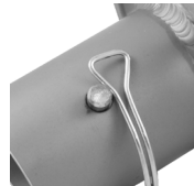
Fig 3 Improperly Secured Leg Coupling Pin
