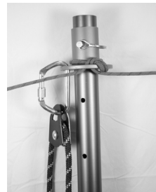
Fig 25 Lash Ring atop of gin pole as main attachment
