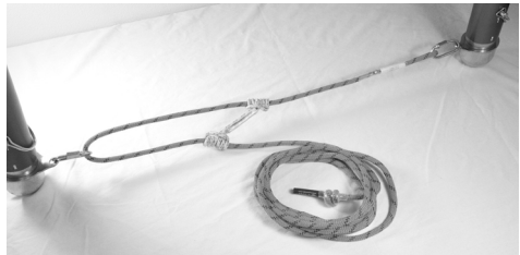
Fig 14 Rope Hobble Loop with Prussic. Sewn loop connected to quick link; large loop connected to 2nd leg quick link.
