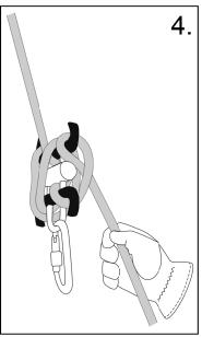
Alternatively, the descender can be tied off by crossing over and securing a half-hitch on the right side horn.
