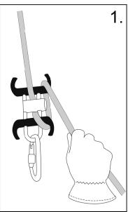
For rappel applications, or for lowering light to moderate loads, the rope should engage the top and bottom horns as shown in the photo.
