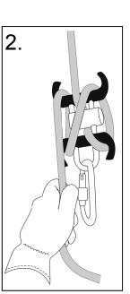
The descender can be tied off by securing a half-hitch around the top horn.
