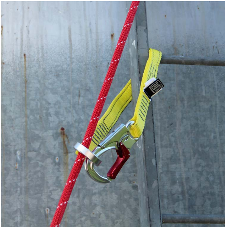
Wrap the lanyard around the structure and connect the carabiner into the ring.
