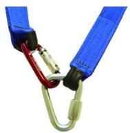
WARNING: the FastLink<sup>™</sup> Anchor Strap should not be used in a Choker configuration as this may put a side load on the carabiner. Ensure the Delta Quick Link and the carabiner are locked and secured prior to loading the system. Care should be taken to make sure that the strap is placed over a surface free of burrs or otherwise sharp features.
