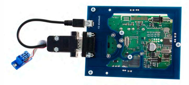
Connect MBProg 2 Click'n Go cable to MBProg. Connect USB cable to MBProg and PC.
