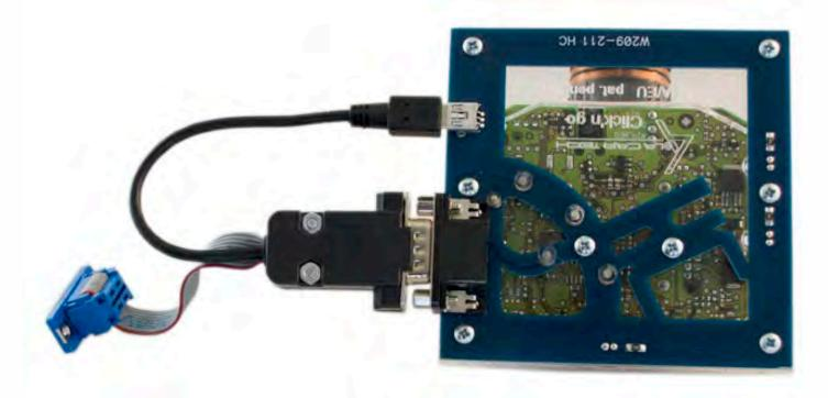
Connect MBProg 2 Click'n Go cable to MBProg. Connect USB cable to MBProg and PC.
