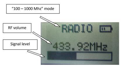
Press any button on remote control. If it sends any radio signal you see the information on the LED screen: RF volume and level of RF signal.
