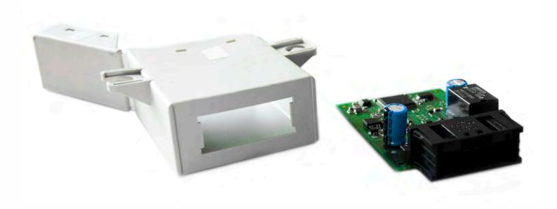
Match EWS4 board top with Click'n Go adapter top. Connector must go over the "Connector" text.
